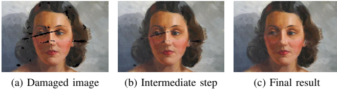
Fig. 2. Progressive nature of a digital inpainting algorithm.
